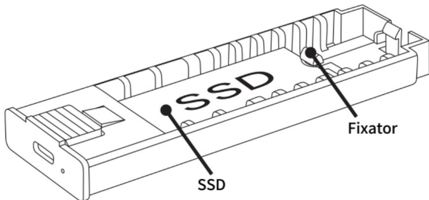
4. Push the inner tray in to the enclosure until the lock catches, then the installation is completed.
