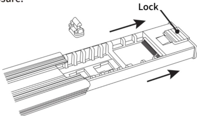
2. According to the length of your SSD, install the accessory fixator to the right place. For 2280 size SSD, there is no need for the fixator.
