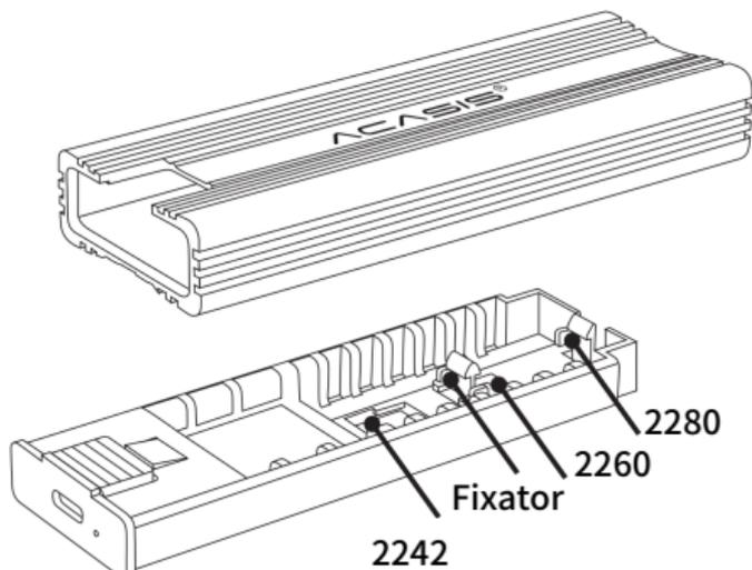
3. At a 45-degree angle, insert your SSD until it is properly seated, then use the fixator to fix SSD.
